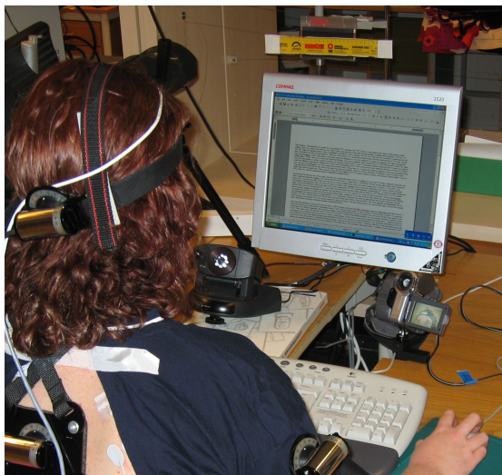
Fig. 2. The video camera used to record eye blinking is seen below and to the left of the VDU-screen
