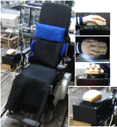
Fig. 3. Description of electric wheelchair with force detecting interface
