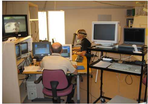
Fig. 1. The test set up, with workplace, glare source, and test person (to the right)
