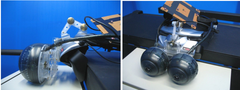
Fig. 4. The eMagin Z800 HMD has been modified by adding two Firewire cameras to capture one image for each eye and an active marker that is used to track the user position. The total weight of this first prototype setup is about 350 grams but it could be reduced in the final setup.
